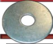
Originally developed for auto body repair, fender washers are large O.D. flat washers that are used extensively in sheet metal, drywall, electrical and plumbing applications where a larger bearing surface is desirable. They are thinner than conventional washers with small holes relative to their large outside diameter. Fender washers are zinc clear plated and are available individually by size or in assortments.
